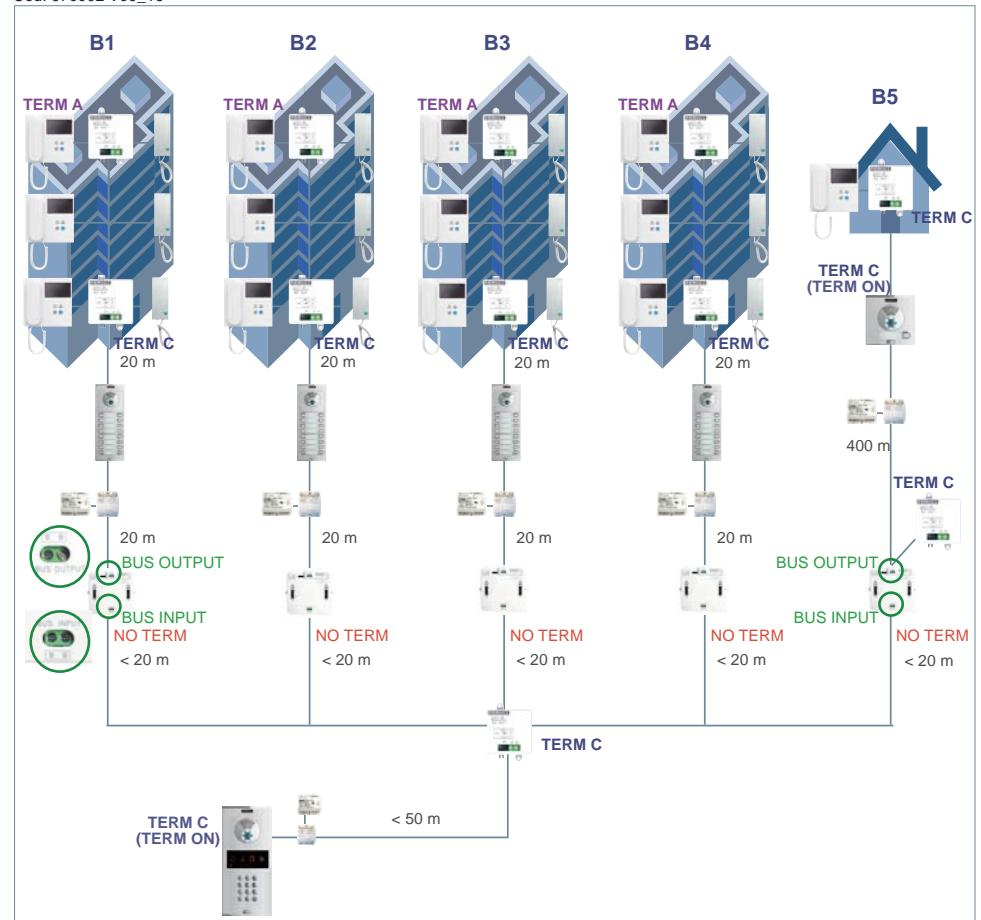
Distancias para cable 2x1mm<sup>2</sup> - Cable distances 2x1mm<sup>2</sup>Câble distances 2x1mm<sup>2</sup> - Kabelstrecken 2x1mm<sup>2</sup>Cabo distâncias 2x1mm<sup>2</sup>
