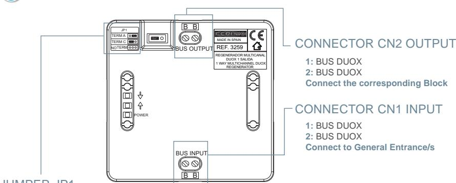
The INPUT terminal must connect to the corresponding installation section of the general entrances and the OUTPUT terminal to the corresponding block (1 multichannel regenerator per block). The INPUT terminal has an adaptation of the incorporated line (configurable via JP1), to take advantage of the termination relative to the installation's topology.
